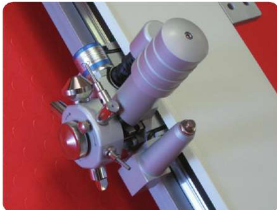
Execution with 6-position revolver to speed up feeler pin change
